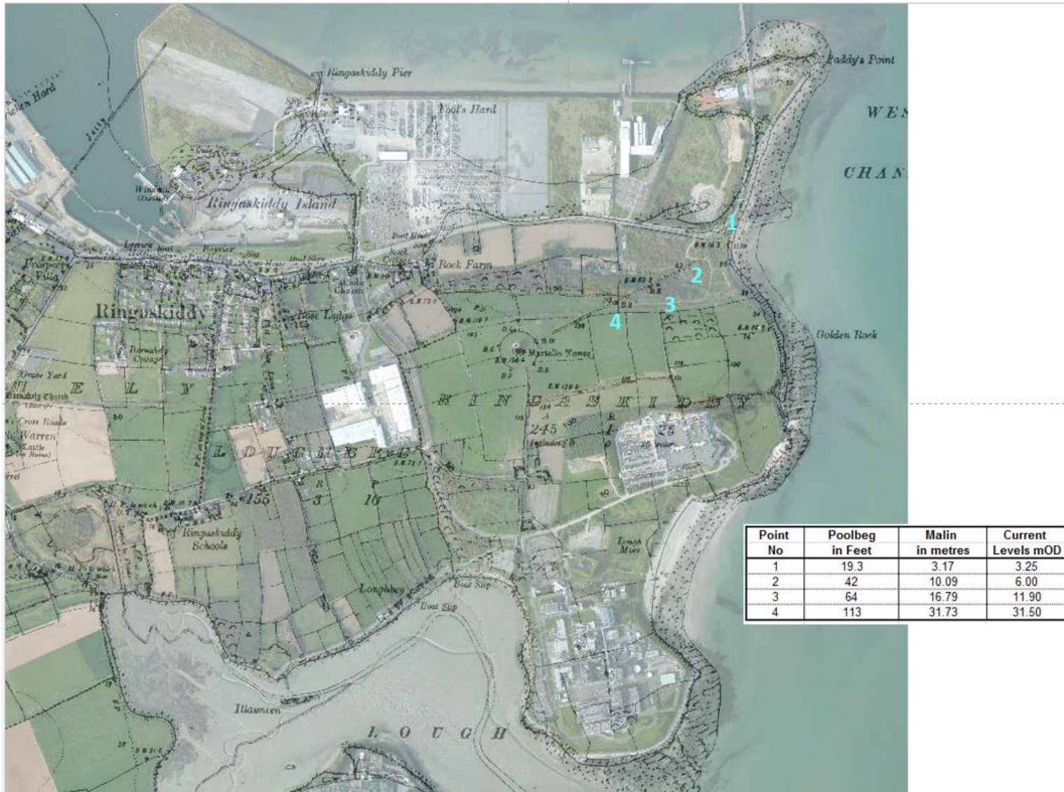
Figure 3a – Ground level changes on site since 1934
